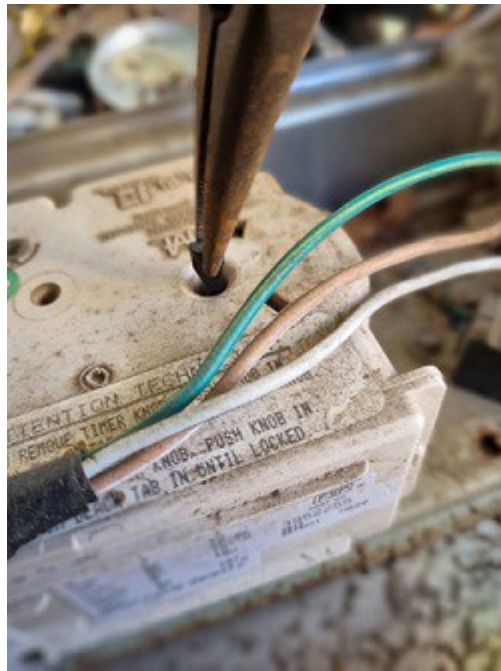
Illustration 1: WP Timer Knob removal, pull the pin out a little
